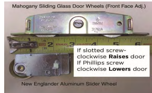
If a mahogany slider, the plastic caps will be on the lower front panel (adjustment area) There are at least two wheels per door. Mahogany wheels # 620-5216 approx. $11 New Englander wheels # 620-3854 approx. $11
